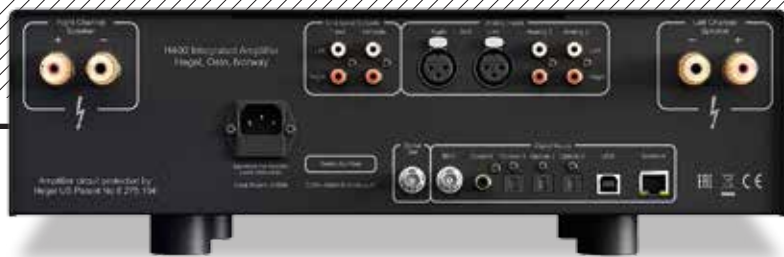
ABOVE: Single 4mm speaker outlets, plus fixed and variable preamp outs are joined by three line ins (one balanced on XLR). The row of digital ins includes three optical, two coaxial (RCA/BNC), USB-B and an Ethernet port. A digital out (BNC) is included
