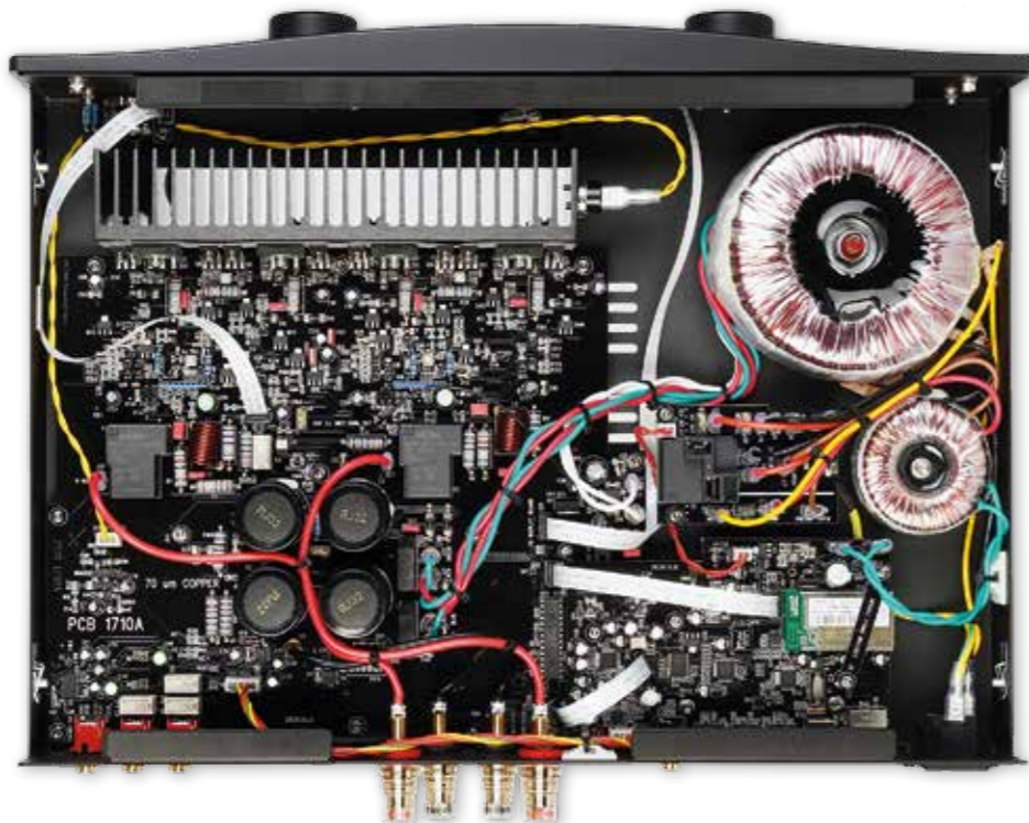
RIGHT: One pair of Sanken power transistors are deployed per channel [heatsinks, top left], fed from a toroidal transformer and linear PSU [right]. Libre-sourced digital board [lower right] offers USB and network access
